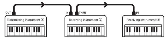
Transmitting instrument ① sends transmit channel and keyboard information to receiving instruments ②/③. The information arrives at the receiving instruments ②/③.
