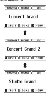
The ◀ or ▶ buttons can also be used to select sounds and cycle through the different sound variations.
