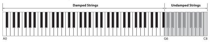
As a result, the strings of these 'undamped' treble notes are free to vibrate in sympathetic resonance with those of lower keys – independently of the damper pedal position – helping to enrich the sound with additional harmonics and tonal colour.
