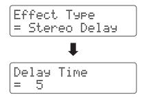
Press the  $\blacktriangledown$  or  $\blacktriangle$  VALUE buttons to adjust the value of the selected effects setting.
