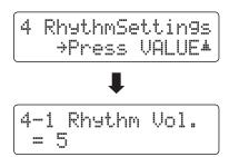
Press the ▼ or ▲ VALUE buttons to adjust the value of the selected Rhythm Section setting.
