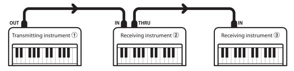
Transmitting instrument ① sends transmit channel and keyboard information to receiving instruments 2/3. The information arrives at the receiving instruments 2/3.
