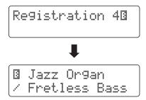
Alternatively, press the  $\blacktriangledown$  or  $\blacktriangle$  VALUE buttons to cycle through all 28 different registration memories.
