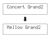
The  $\blacktriangledown$  or  $\blacktriangle$  VALUE buttons can also be used to select sounds, and cycle through the different sound variations.
